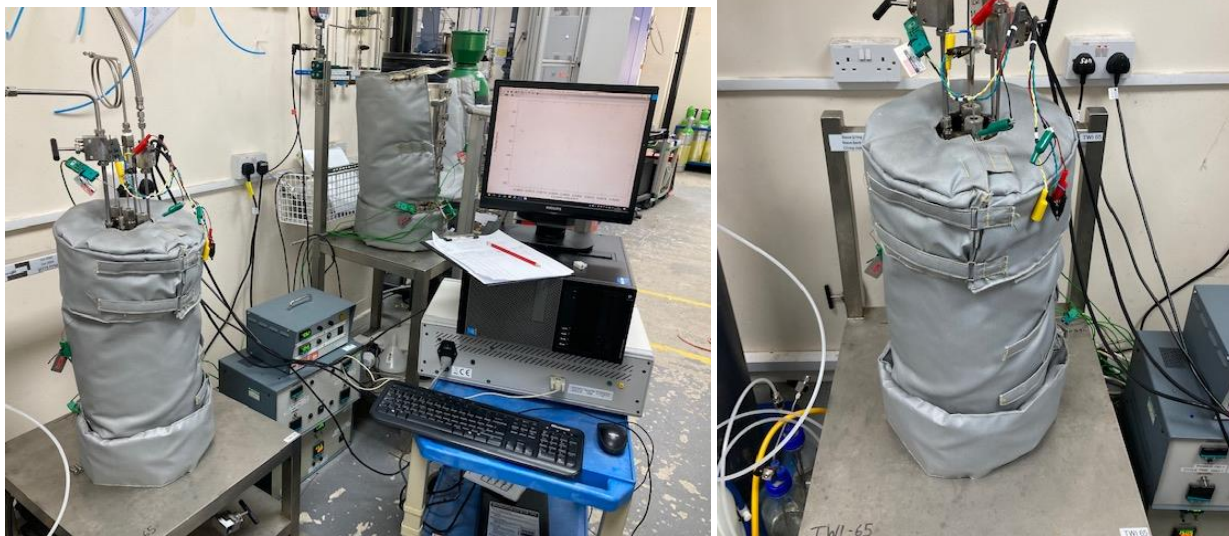
Figure 8 Photographs of the 120°C electrochemical testing setup
