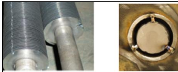
Figure 4. Carbon steel tubes with circular helical aluminium fins and cylindrical insert used as cross-sectional area reducer
