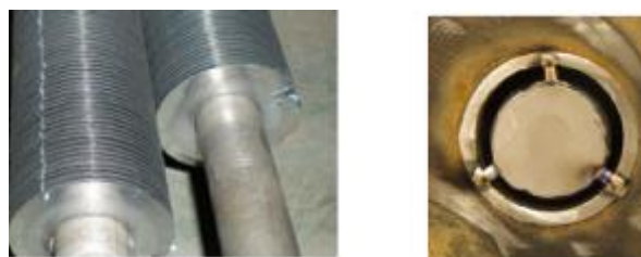
Figure 37. Carbon steel tubes with circular helical aluminium fins and cylindrical insert used as cross-sectional area reducer
