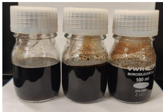
Figure 6. Aged adipic acid samples after 1000 h at 165 °C
