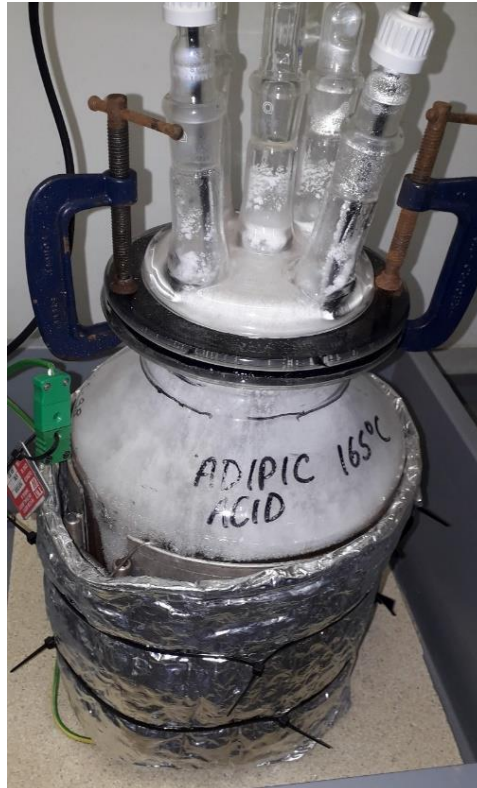
Figure 7. Glass reactor during tests, showing that high partial pressure led to a solidification of the vapour on the upper part of the vessel and the lid
